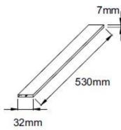
Epoxy resin UL:94V-0
